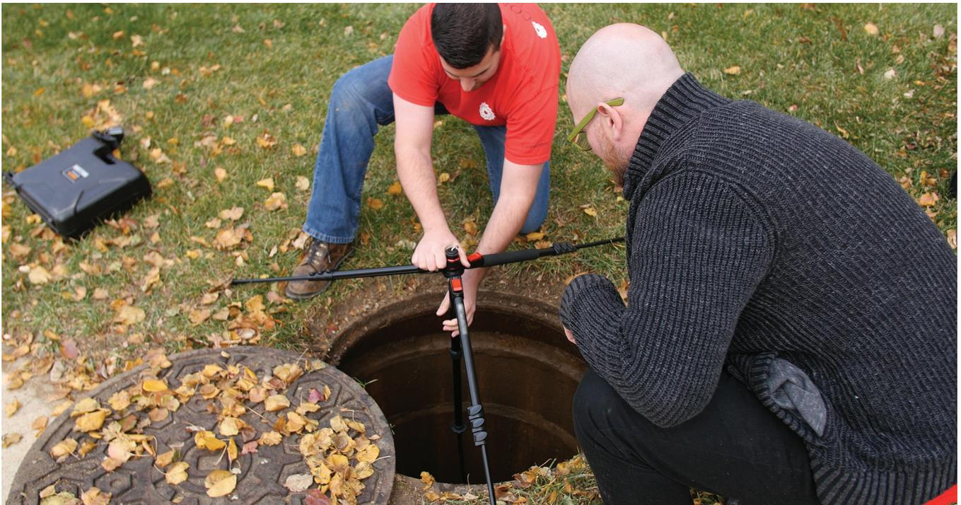
A survey of a manhole may uncover air-quality dangers, which would immediately halt the audit process and leave spaces undocumented. The IVaaS solution includes an assessment of the site, which allows for confined spaces to be evaluated safely, without descent; this “heads-up” approach to surveying means deeper-dive survey activities can be planned with confidence.
